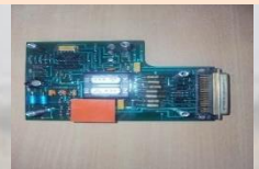
Sea King RADAR PCBs Modules
