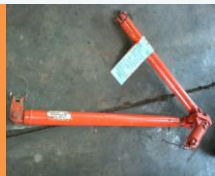
Lifting and Jacking Truss
