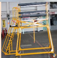
SECTION 48 ACCESS PLATFORM
