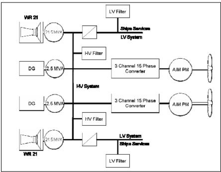
Fig 4. Integrated Electric Propulsion (viz., IEP/ IFEP) Configuration
