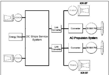
Fig 3. All-Electric-Propulsion (AEP) System Configuration
