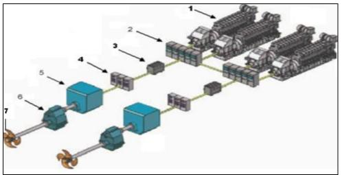
Fig 1. A typical Schematic Layout of an Electric Propulsion System: (1) Prime Mover (2) Switchboards (3) Convertors (4) Harmonic Filters (5) Pulse Frequency modulators (6) Electric Propulsion Motors (EPMs) (7) Propulsors (Pods/ Shaftless-Rim-Driven Propellers)
