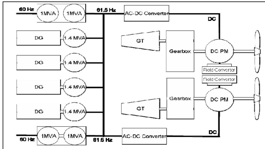
Fig 2. An example of Hybrid Electric Propulsion viz., CODLAG Configuration
