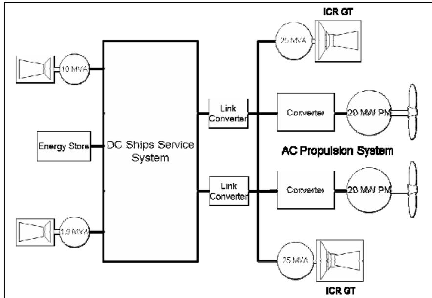
Fig 3. All-Electric-Propulsion (AEP) System Configuration
