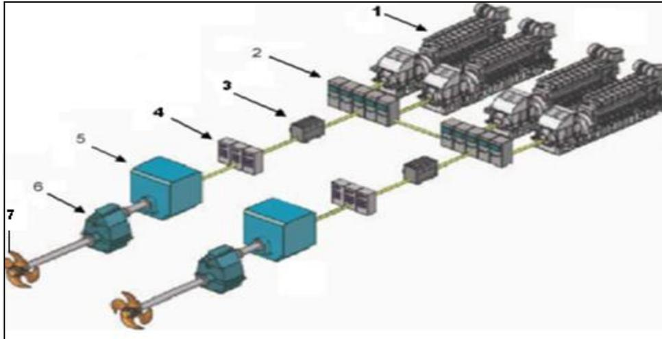
Fig 1. A typical Schematic Layout of an Electric Propulsion System: (1) Prime Mover (2) Switchboards (3) Converters (4) Harmonic Filters (5) Pulse Frequency modulators (6) Electric Propulsion Motors (EPMs) (7) Propulsors (Pods/ Shaftless-Rim-Driven Propellers)
