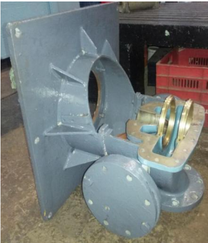
Fig. 10 Recovered Pump after Cold Weld Repairs
