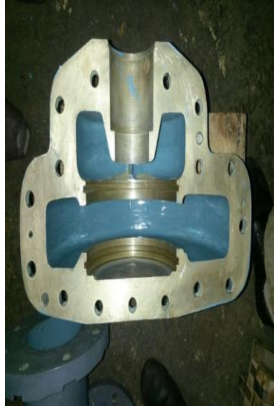
Fig. 9 Condition of Pump Post Surface Preparation and Internal Coating
