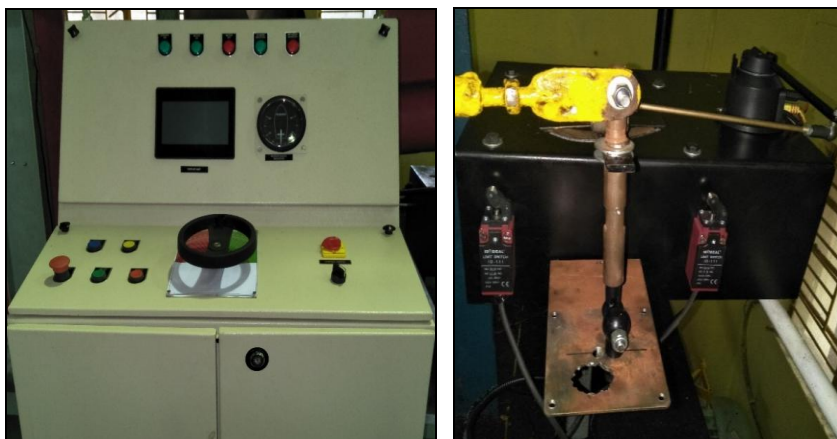
Fig. 4 Steering Gear Setup with PLC based Control Panel
