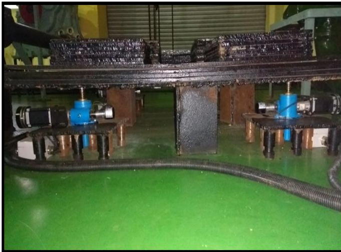
Fig. 3 Designed Cradle Lifting Mechanism
