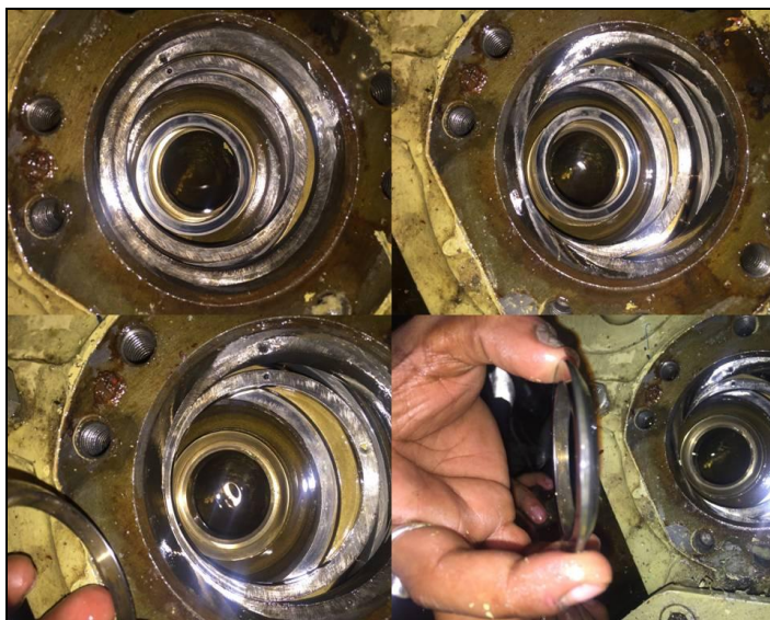
Fig. 9 Scoring Marks on the Surface of Metallic Rings and Conical Washers
