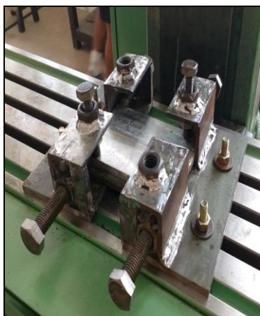
Fig. 8 Fixture Mounted on The Table of VMM (Top)
