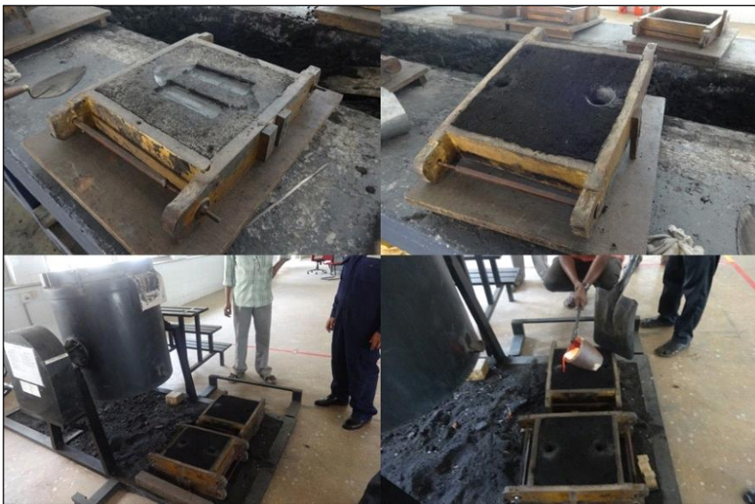
Fig. 2 Mould Preparation and Casting of Aluminum Plates at the Foundry Shop
