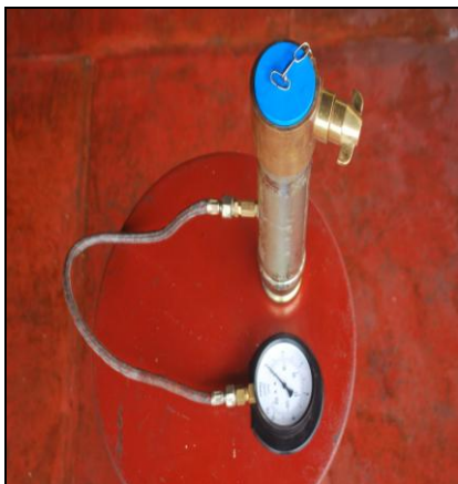
Fig. 1 Auto Coupling System for Measuring Discharge Pressure of Submersible Pump
